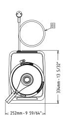
Electric Supply voltage: 220-240 V/1N ph/50/60 Hz Electrical power, max: 0.75 kW 0.75 kW **Total Watts:** Capacity: Performance (up to): Capacity: 3.6 litres Key Information: External dimensions, Width: 252 mm External dimensions, 334 mm Depth: External dimensions, Height: 476 mm **Shipping weight:** 19 kg Meat mincing capacity: 0 kg Mayonnaise preparation 0 kg capacity: Pastry preparation capacity: 0 kg
